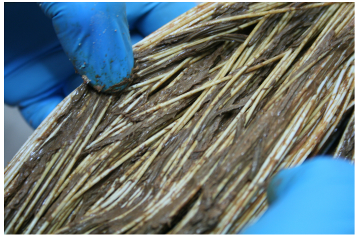
Heavy silt, iron and biological fouling.
